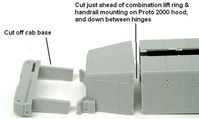
6. Remove about 1/3 of the material from the rear of the rearmost tabs that supported the exhaust stack section, since you may need to do some filing in this area later, and it is easier to remove part of these tabs now to allow working room.
