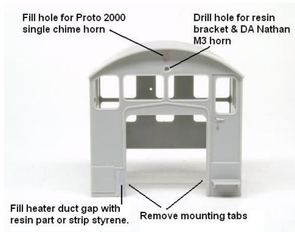
15. File or cut off the small mounting tab inside the heater duct cutout on the front wall of the cab. This tab fits into the hole on the cab base that you removed in the previous step. It is no longer needed, and would interfere with the installation of the resin parts.
