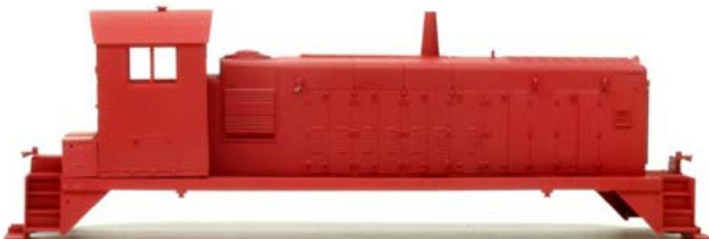
29. Glue the fan housing in place. Note that there is cast-on fan detail that will be covered by the resin fan housing. This detail is provided in case you want to use a see-through fan housing from a Highliners F7 or a Life Like SD-7, SD-9, or E-8.
